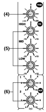
subtract from the mix. Cutting the HIGH control can reduce unwanted hiss during multi-track recording, while attenuating the MID or LOW can eliminate feedback in a live performance or clear up a muddy sounding mix.
